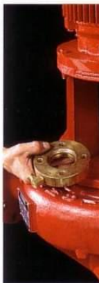
3) Disconnect seal plate bolts. The seal plate can then be taken out. With inside seal removed, follow
